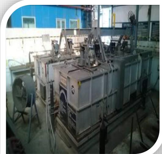
Spherodizing & Annealing Machines
