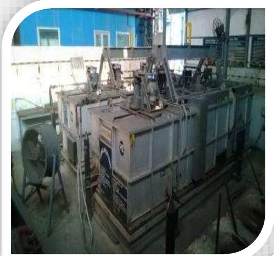
Spherodizing & Annealing Machines
