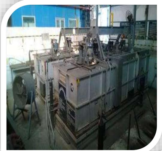
Spherodizing & Annealing Machines
